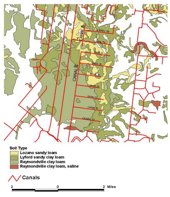
Figure A-1. Canals in the project area overlaid onto the soil series map.
