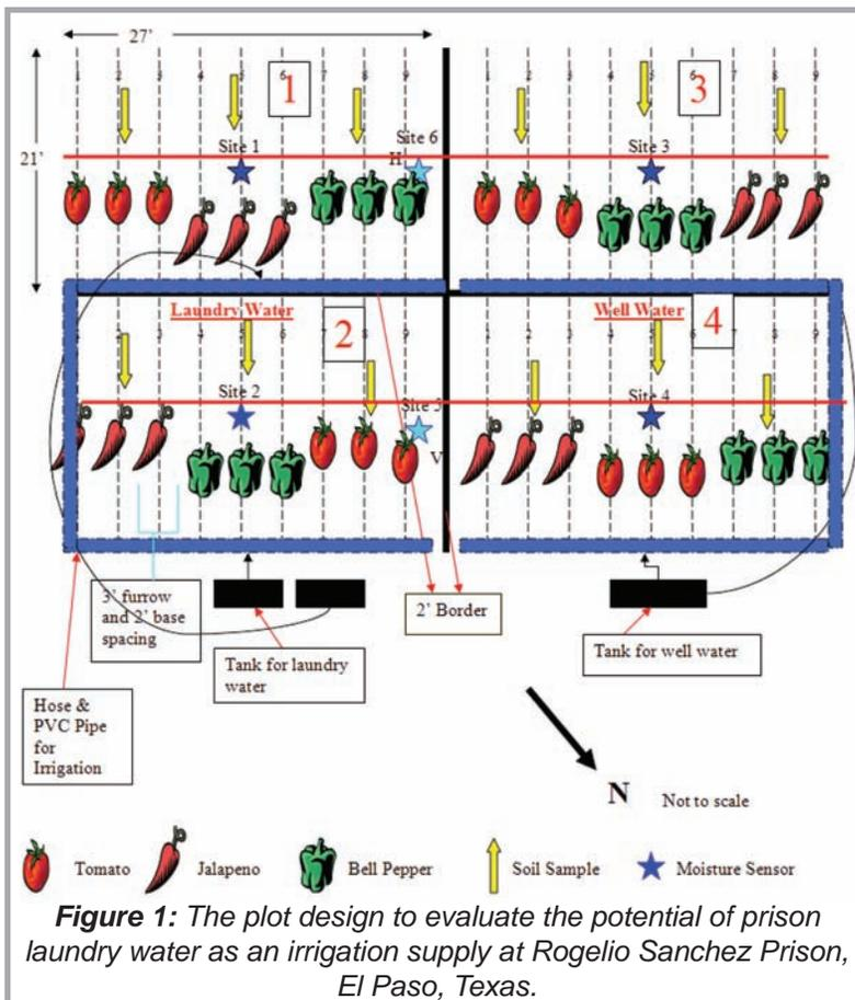
**Figure 1:** The plot design to evaluate the potential of prison laundry water as an irrigation supply at Rogelio Sanchez Prison, El Paso, Texas.
