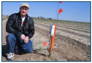
Dr. Shad D. Nelson, associate professor of agronomy and horticulture at Texas A&M University-Kingsville, monitors water depletion in an ADI grower's drip irrigated onion field using realtime ECH2O EC-10 soil moisture sensors and automatic Em50 data loggers manufactured by Decagon Devices, Inc.
